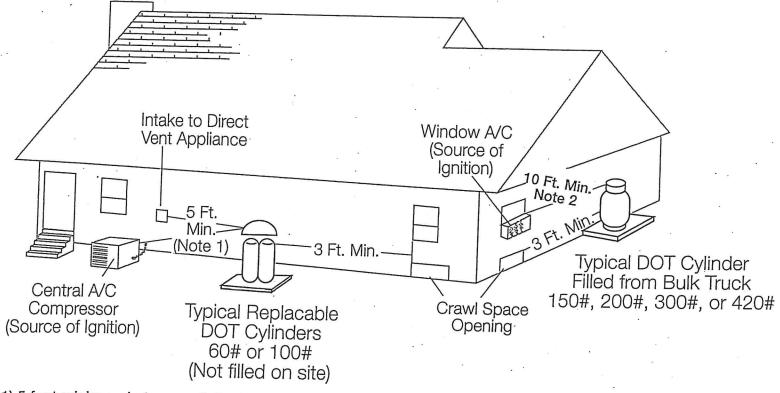
Notes: 1) 5 foot minimum between relief valve discharge and external source of ignition (air conditioner), direct vent, or mechanical ventilation system. (attic fan).
